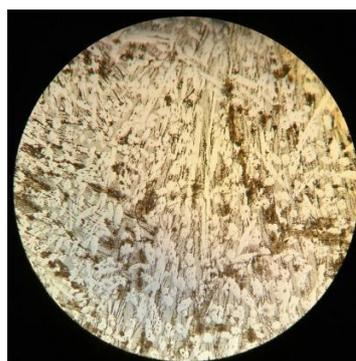
Figure 1.6. Microstructure of C12 steel.
