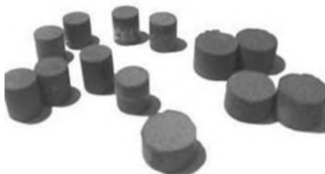
Figure 1. Briquettes of furnace mono-charges based on 6-8% exclay
