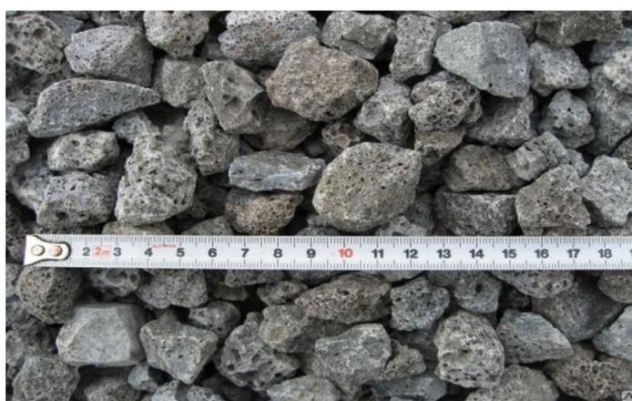
Figure 1. Samples of road-building crushed stone from blast furnace slag of a fraction of 20-40 mm
