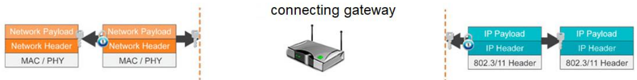
Figure 2 – Packet routing to an IP network in the absence of IP protocol support (ZigBee, Bluetooth LE, ANT/ANT+)
