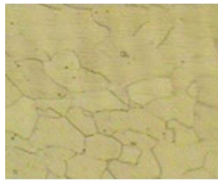
Figure 3. Microstructure of strip rolled as per mode B ( \times 1000 )
