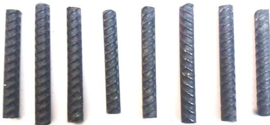
Figure 5. Obtained experimental samples of reinforcing steel profile №12
