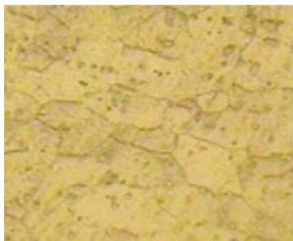
Figure 2. Microstructure of strip rolled as per mode A ( \times 1000 )
